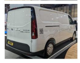
Info: The new Maxus eDeliver 7 is the third model in the firm's rapidly expanding electric van line-up. The battery capacity could be 77 o 88kWh and develops a power of 150kw (204Hp). The autonomy is located at 360km according to the WLTP cycle.
