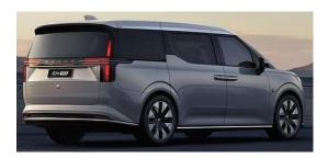
Info: The new EM90 is the result of strategic collaborations being carried out by the different car brands that are part of the Geely automotive conglomerate, specially from ZEEKR and its Zeekr 009 which brings Volvo's first electric minivan. It has a battery capacity of 116kWh and develops a power of 197kw (268Hp). The autonomy is located at 738km according to the CLTC cycle. Rivals of the new Volvo EM90 are models like the Volkswagen ID.BUZZ, Lexus LM, Maxus MIFA 9 and the ZEEKR 009 itself.
